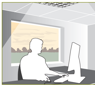
PERSON PRESENT. INSUFFICIENT DAYLIGHT. LIGHTS ON.
